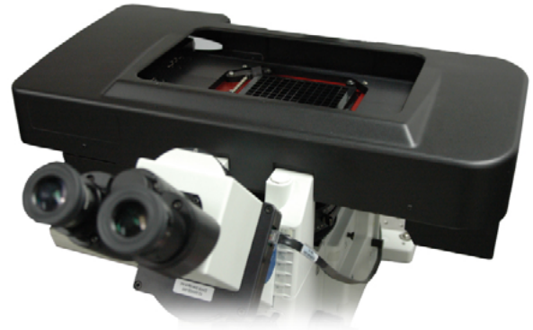
Figure 1: DeltaVision's Microtiter Stage
